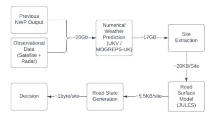
Figure 1: Visualisation of data flows in the production of a road state forecast.
