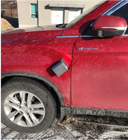
Figure 2 Pavement temperature sensor.
