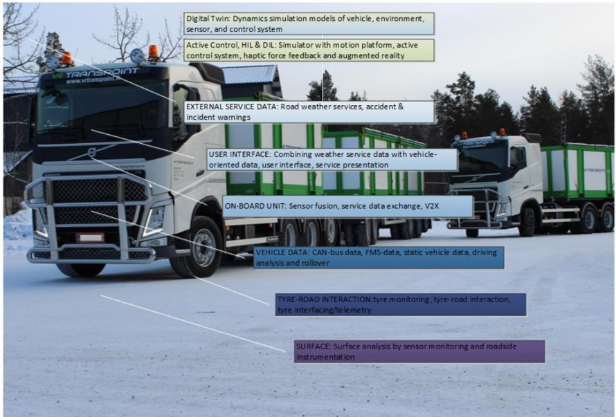
Fig. 2. SafeTrucks system architecture.
