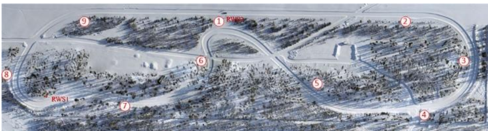
Fig. 1. Sod5G test track. The Road Weather Stations are marked as RWS1 and RWS2, IoT weather sensors as numbers 1-9.
