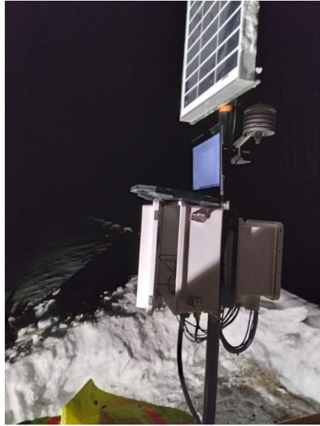
Fig. 3: Installation of mini-RWIS system at Chena Hot Springs Road MP 10 on January 21, 2021. Left: pole-mounting with solar module and weather sensors. Right: mini-RWIS data logger mounted on pole.
