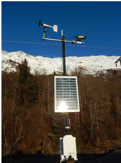
Fig. 1. mini-RWIS stations are self-sufficient, running exclusively on solar power and batteries to allow them to be placed anywhere you need them, regardless of existing infrastructure. They are easy to integrate, featuring embedded cell communication as well as NTCIP / Datex2 / Modbus compliance, making integration into an existing RWIS network simple.
