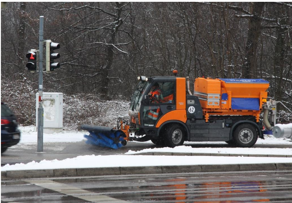
Fig. 2 - Narrow gauge vehicle with front sweeping broom and spreader for pre-wetted salt treatment [picture source Cypra, 2021]
