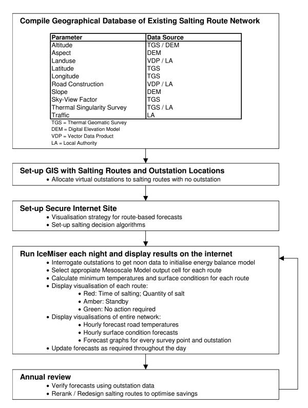
Figure 1 Flow diagram showing the procedure in developing XRWIS
