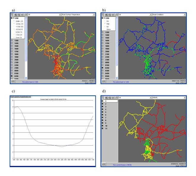
**Figure 2** Conceptual visualisation of the new XRWIS paradigm showing a) Road Surface Temperatures, b) Road surface Conditions, c) Forecast Graph and d) 'Traffic light' salting routes.
