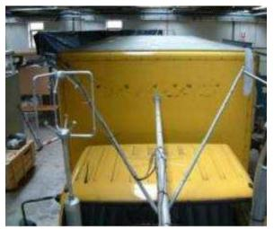
Figure 6:Front view. Front tapping points, anemometer
