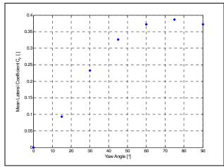
Fig. 3: Aerodynamic coefficient of the lateral force
