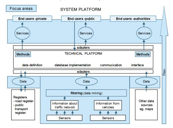
Figure 1. Main principles of ROADIDEA service system platform and the use of methods to be developed.
