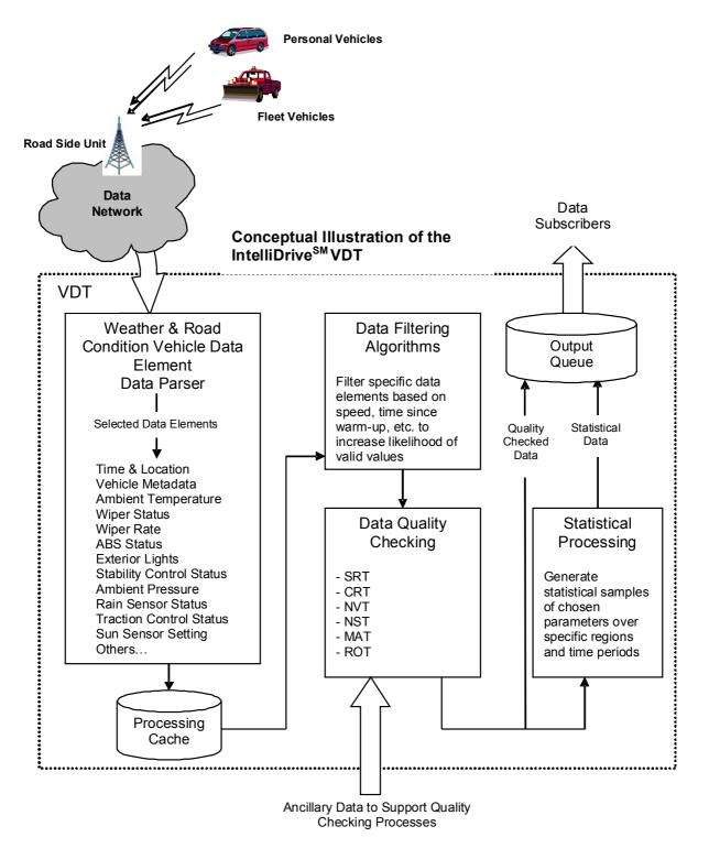
Figure 1 - Vehicle Data Translator (VDT) Conceptual Illustration
