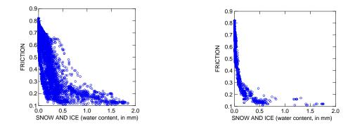
Figure 7. Scatter plot of friction vs. the sum of snow and ice (water content in mm) on the road. Based on DSC111 observations in Utti (in southeastern Finland) during winter 2007/08. The left figure includes all observations, the right figure covers those cases when road surface temperature was below  $-5^{\circ}C$  (data source: the Finnish Road Administration).
