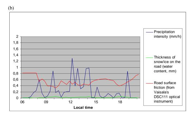
Figure 6. Road weather observations at Vaskisalmi station (about 4 km west of Helsinki city center) on 8 February 2007 06-20 local time: (a) air, road surface and dew point temperatures, (b) precipitation intensity, thickness of snow/ice on the road as well as road surface friction measured by Vaisala's DSC111 optical instrument (data source: the Finnish Road Administration).
