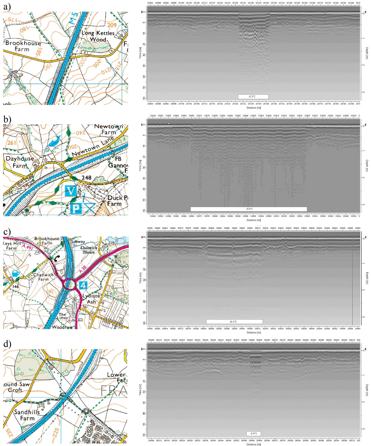
Figure 4: Location, radargrams and typical magnitude of the thermal singularity (under stable conditions) of four bridge decks on the study route. ©Crown Copyright/database right 2009. An Ordnance Survey/Digimap supplied service
