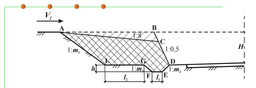
Formula of calculation quantity of snow deposits on the road surface of closed ditches
