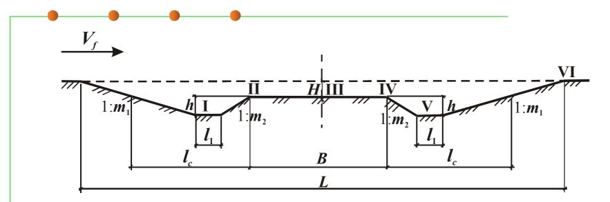
Formula of calculation quantity of snow deposits on the road surface of open ditches
