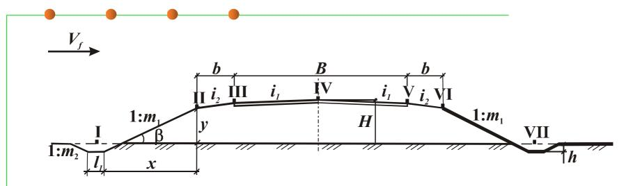
Formula of calculation quantity of snow deposits on the road surface of embankments
