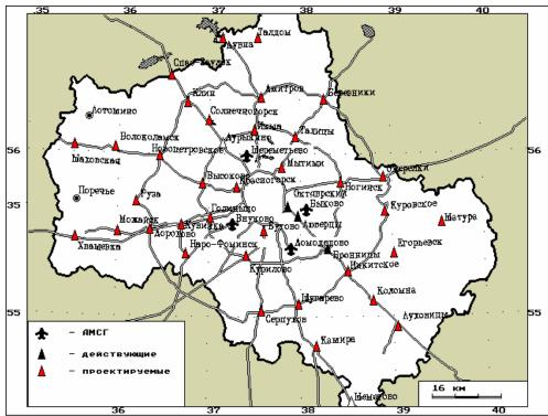
Fig. 5.1. Proposed efficient pattern of RWS arrangement (red triangles) over Moscow Region.
