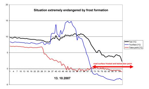
Figure 5. Estimation of icing danger during the actual measured period.
