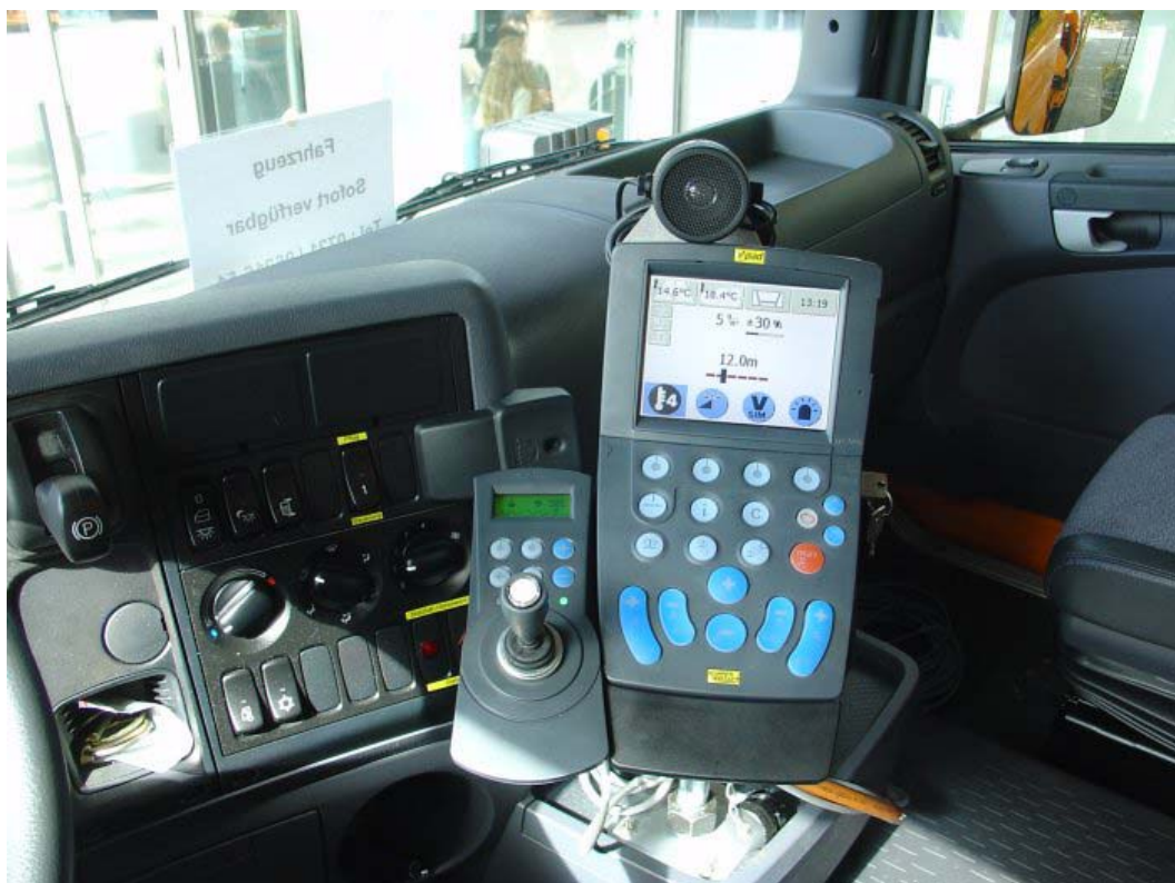
Fig. 8 Control panel to control spreaders and snow plows with integrated data recording and route guidance
