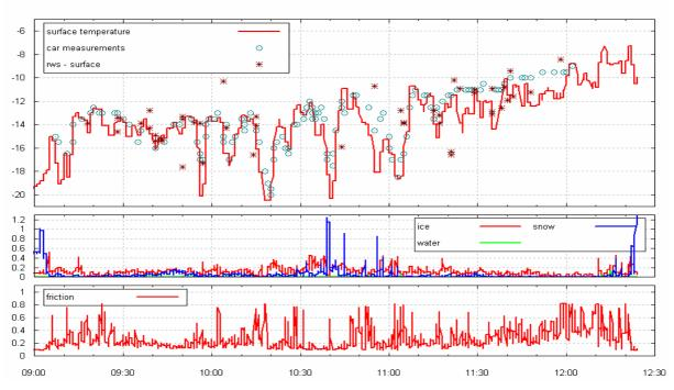
Fig. 7. Road weather measurements 30.1.2007 presented as a function of time and distance. On the top: Road surface temperature (line mobile measurements, stars road weather station, circles car measurements). In the middle: Thickness of water, ice and ice layers in mm:s. On the bottom: Value of friction.
