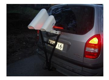
Fig. 6. Mobile measurement devices attached to the vehicle.
