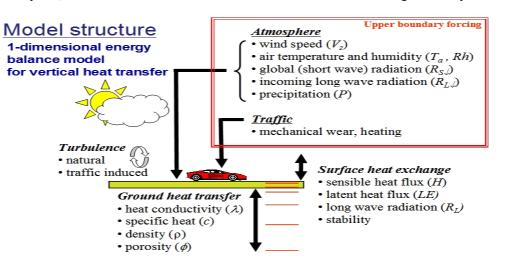
Figure 2. Schematic of the road weather model.
