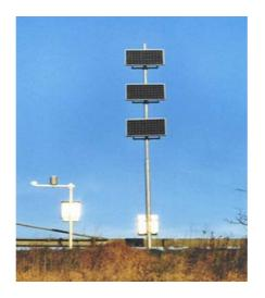
Fig. 5. Measuring station with solar cells and wireless transmission
