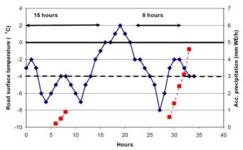
Figure 1. Figure to explain the counting of hours favourable for using the warm wetted sand method.
