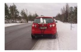
Fig. 2 DSC111 and DST111 installed for mobile measurements
