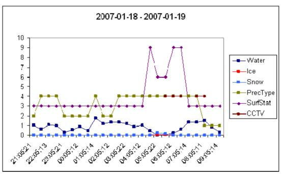
Fig. 4. Road weather conditions change measured by different devices on 18-19th of January, 2007.
