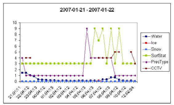
Fig. 5. Road weather conditions change measured by different devices on 21-22<sup>nd</sup> of January, 2007.
