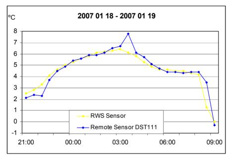
Fig. 8. Road weather temperature change measured by two sensors on 18-19th of January, 2007.
