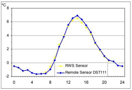
Fig. 7. Averaged daily road surface temperature fluctuation.
