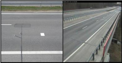
Fig. 2. The spot of remote sensor (white square) on the left and visual range of RVC on the right.
