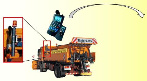
Example: the **Thermomat** from Küpper-Weisser (Pavement temperature measurement)
