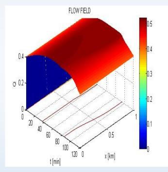
Parameters: vo=130 km/h; Qmax=1875 veh/h
