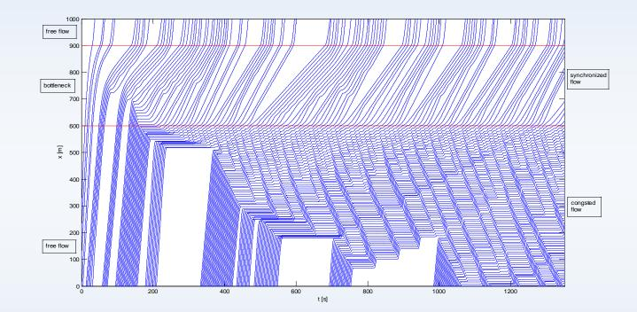
The goal: Macro-modeling based on fundamental diagram of flow and continuity equation. Boundary condition is determined by the predicted flow
