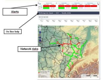
Figure 7 : Road weather risk interface (red : a threshold is exceeded, green : no risk)
