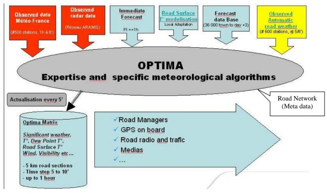
Figure 1 : Optima synthetic diagram
