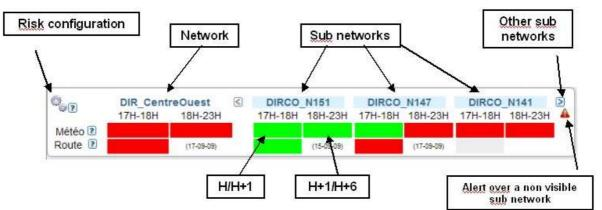
Figure 8 : The alerts are resumed in a banner on the top of the Optima's interface
