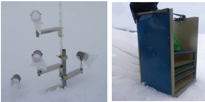
Figure 1: Cylindrical net-type blowing-snow trap meters (left) and a box-shaped net-type blowing-snow trap meter (right)
