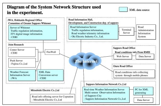
Figure 1. Diagram of the system network structure used in the experiment
