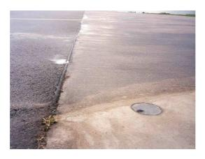
Figure 6: Water film sensor and the surrounding paved area. The sensor has dried-up even though the paved area is still moist.
