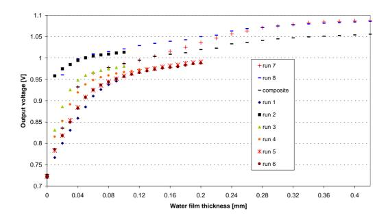
Figure 1: Calibration curves for the water film sensor.
