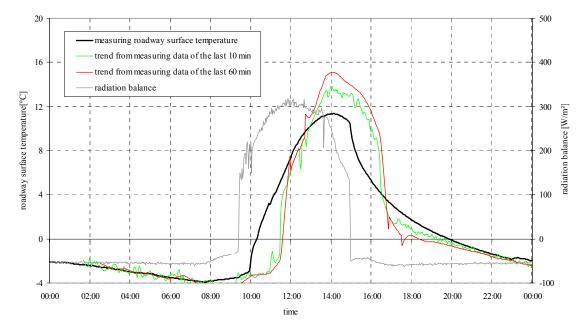
Figure 1: Actual and calculated roadway surface temperature progression over 24 hours on a largely cloudless day (mid-January)
