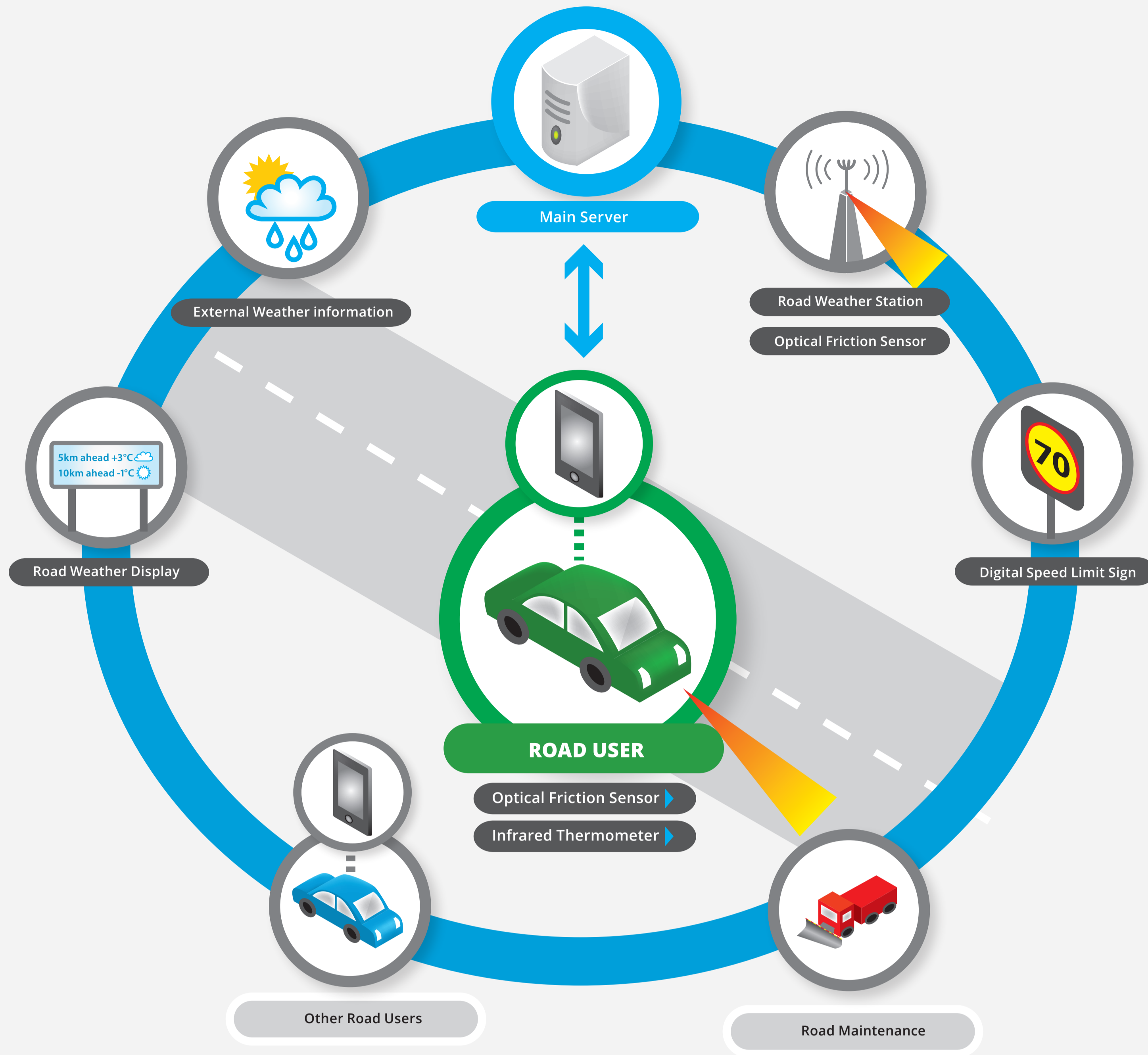
Visualization of road condition and friction data in a public web interface by using different in-vehicle sensors
