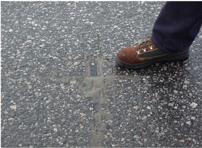
Passive sensors do not interfere with the measurement area
