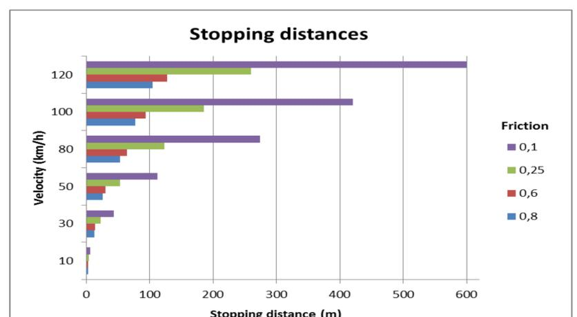
Stopping distances (including reaction distance when reaction time is 1 second and braking distance) as a function of different velocities and frictions.
