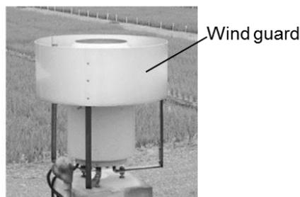
Figure 1 Heated tipping bucket precipitation gauge with wind guard (Hokkaido type gauge)
