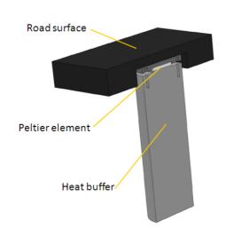
Figure 4: Cooling element used in Passive-BIRDS
