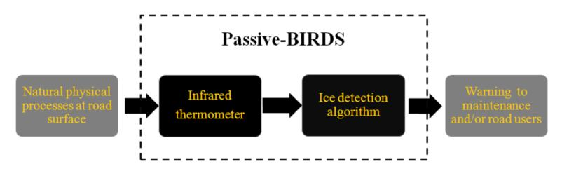
Figure 2: Schematic overview of the process chain involved in Passive-BIRDS
