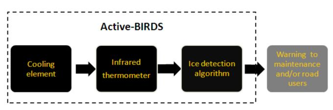
Figure 3: Schematic overview of the process chain involved in Active-BIRDS
