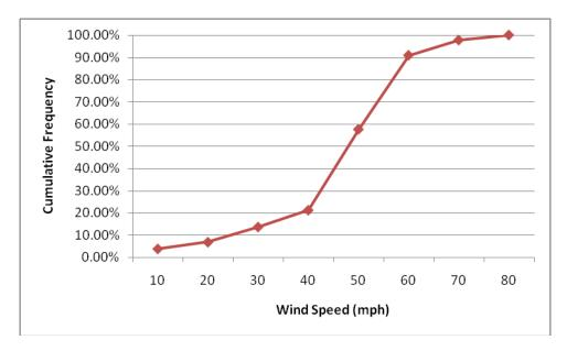
Figure 3. Cumulative Crash Frequncy of Wind Speed When Crash Occurred
