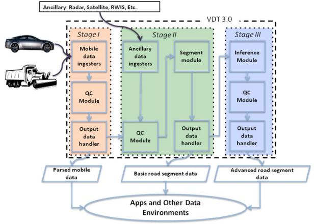
The VDT is engineered in a modular way. Figure 1 is a high-level schematic of the design of VDT 3.0.
