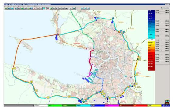
Figure 5. Road surface temperature, condition and precipitation forecast for the highway ring.
