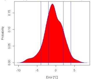
Figure 5. Probability distribution for RST prediction errors (= predicted values – measured values) for RWS *Verd*. Vertical lines represent abscissa values at -4, -2, 2 and 4.
