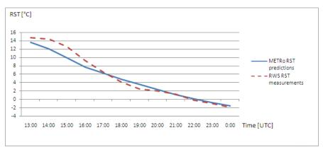
Figure 7. RST predictions calculated at 12:00 and RST measurements at the RWS *Sava Šentjakob* on 18 February 2012. RMS error for RST was 1.25°C.
