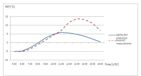
Figure 6. RST predictions calculated at 04:00 and RST measurements at the RWS *Šentožbolt* on 18 February 2012. RMS error for the RST was 5.39°C.
