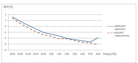
Figure 8. RST predictions calculated at 18:00 and RST measurements at the RWS *Slatina* on 18 February 2012. RMS error for RST was 0.48°C.
