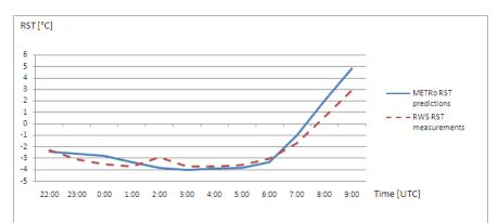
Figure 9. RST predictions calculated at 21:00 and RST measurements at the RWS *Šumljak* on 16 February 2012. RMS error for RST was 0.82°C.
