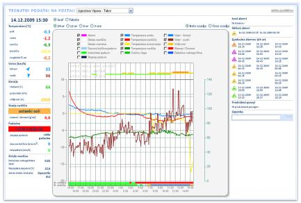
Figure 2. RWIS in Slovenia: detailed overview of events at a chosen RWS. [Source: DARS d.d.]
