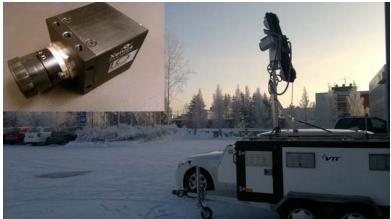
Figure 1: Road side unit (RSU) with Xenics XS-1265 NIR camera. All the test images were capture with this unit. Vehicle on background was carrying stereo camera unit.
