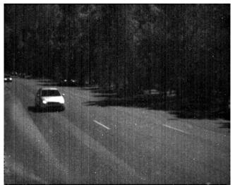
Figure 6: Example of real lane monitoring situation at summer time (dry road). In this case bypassing vehicles caused false detections but these can be filtered in final analysis.
