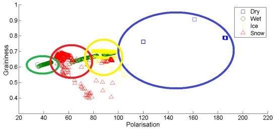
Figure 5: Final classification borders for dry, wet, snowy and icy road surface. The graininess and polarisation parameters can be used in a classifier which is able to separate four different road surface conditions: dry, wet, ice or snow. Note that the wet, ice and snow surface values overlap because they all contain water which is detected by the NIR camera
