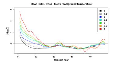
Figure 4. Mean RMSE INCA-METRo road/ground temperature error for different thresholds and lead times.
