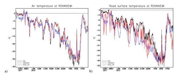
Figure 4. Observed (black line) and modelled by HARMONIE/SURFEX (blue) and FMI's road weather model (red) temperatures on Rovaniemi. Air temperature on the left (a) and road surface temperature on the right (b).
