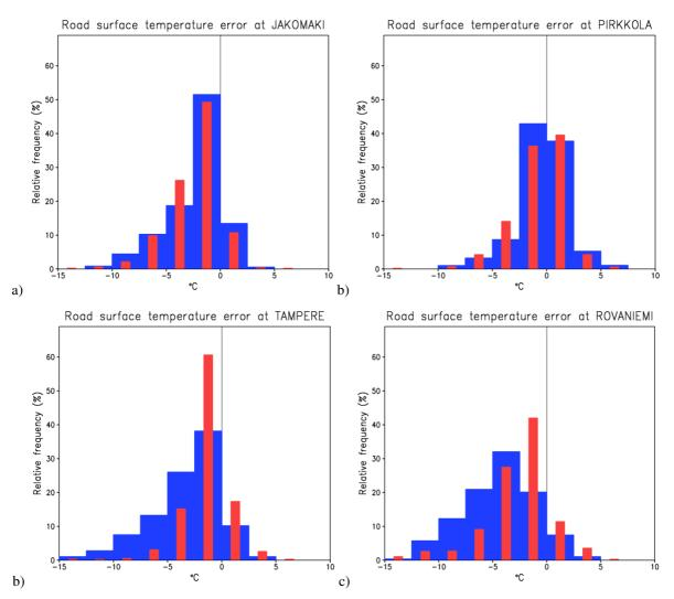
Figure 4. Road surface temperature error between modelled and observed values in four studied places; Jakomäki, Helisnki (a), Pirkkola, Helsinki (b), Tampere (c) and Rovaniemi (d), respectively. Blue colums are presenting HARMONIE/SURFEX and red columns FMI's road weather model.
