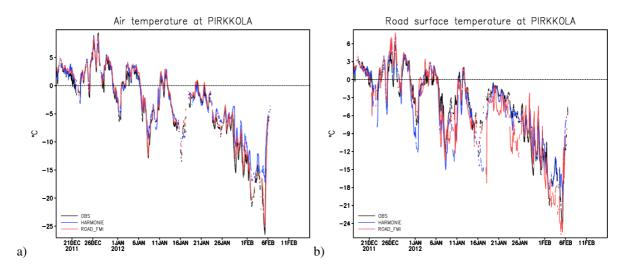
Figure 2. Observed (black line) and modelled by HARMONIE (blue line) and FMI's road weather model (red) temperatures on Pirkkola, Helsinki. Air temperature on the left (a) and road surface temperature on the right (b).
