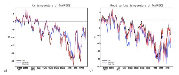
Figure 3. Observed (black line) and modelled by HARMONIE (blue) and FMI's road weather model (red) temperatures on Tampere. Air temperature on the left (a) and road surface temperature on the right (b).
