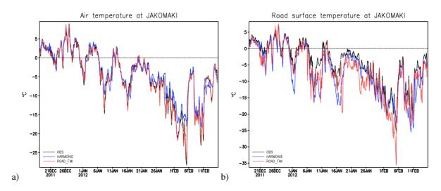
Figure 1. Observed (black line) and modelled by HARMONIE (blue) and FMI's road weather model (red) temperatures on Jakomäki, Helsinki. Air temperature on the left (a) and road surface temperature on the right (b).
