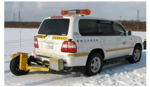
Figure 5. Continuous friction tester (CFT)
