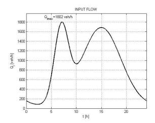
Figure 2. Analytically described dependence of the predicted traffic flow rate Q on time t. Data correspond to the flow on a single lane as forecast by the intelligent module and shown by the graphic user interface in Fig.1.
