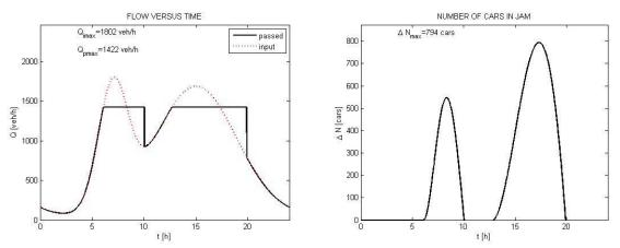
Figure 6. Dependence of the passed flow Q and the estimated number of cars in jam  $\Delta N$  on time t.
