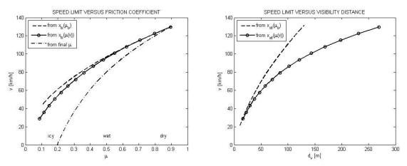
Figure 5. Dependence of the proper speed limit on friction coefficient (left) and visibility distance (right).
