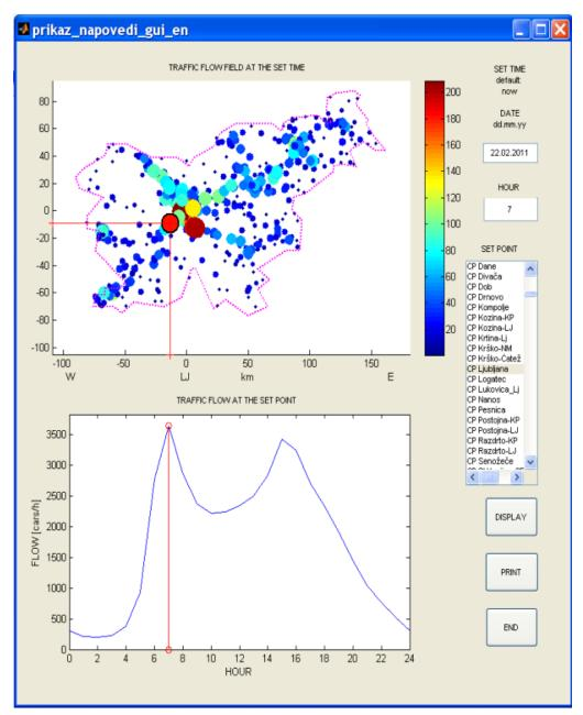
Figure 1 - The graphic user interface of the intelligent module for traffic flow forecasting. The top graph shows the distribution of the predicted traffic flow rate Q(x) in Slovenia at set time, while the bottom one shows the dependence of Q(t) at the selected position denoted by vertical and horizontal line in the top diagram. The radius of the circle at a point in this diagram indicates the value of flow rate at the time of forecasting.
