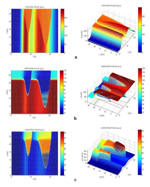
Figure 7. Distributions of traffic field variables: (a) flow rate, (b) velocity, (c) density. Left – ground plan, right – side view.
