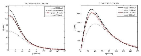
Figure 3. Dependence of velocity v and traffic flow rate Q on the density of cars  $\rho$ . Experimental data are taken from the ref. [5].
