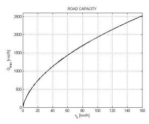
Figure 4. Dependence of the road capacity  $Q_m$  on the speed limit  $v_o$ .
