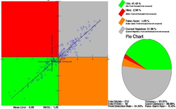
Figure 4. Operational verification scatter-graph of forecast against observed road surface temperatures.
