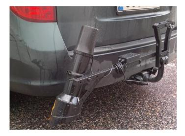
Figure 2. RCM411 installed to a passenger vehicle equipped with a 50 mm trailer ball joint.
