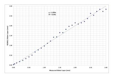
Figure 6. RCM411 performance in measuring thickness of water layer.
