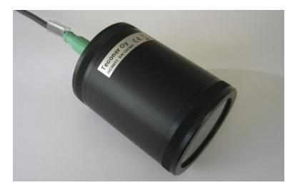
Figure 1. The sensor of RCM411 with the sensor window shown on the lower right corner.
