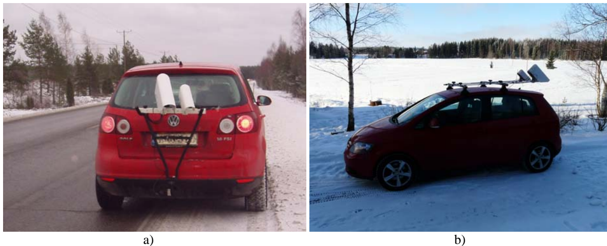
Figure 2. a) The first installation in 2006 using optical remote sensors Vaisala DSC111 and DST111 behind the observing vehicle. b) The second installation on top of the car during ROADIDEA project in 2007-2010.
