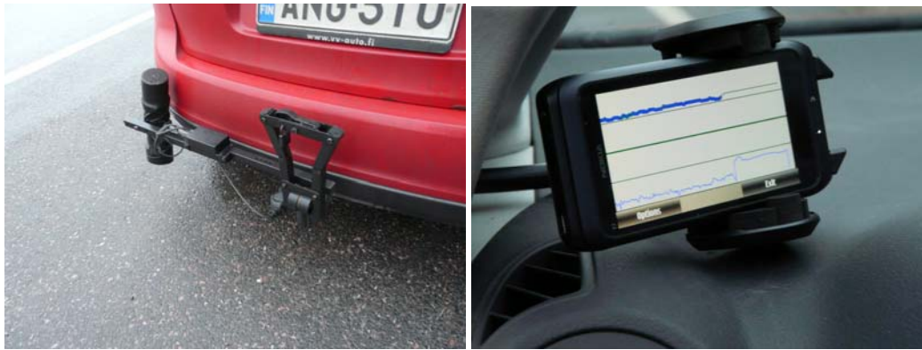
Figure 4. Most recent installation in 2011-2012 using Teconer RCM411.
