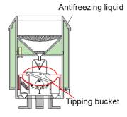
Figure 1 Heated tipping bucket precipitation gauge with wind guard (Hokkaido type gauge)
