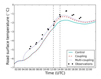
Figure 2. Road surface temperatures for 18<sup>th</sup> December 2015 forecast runs for the point nearest to the red start point of Figure 1. The control run is shown with cyan continuous line, the run with simple coupling with red dashed line, and the multi-coupling run with blue dotted line. Black dots are mobile observations. The left vertical line at 12:00 noon shows the start of HARMONIE forecast, and the right one the end of the last coupling period of the multi-coupling model run.
