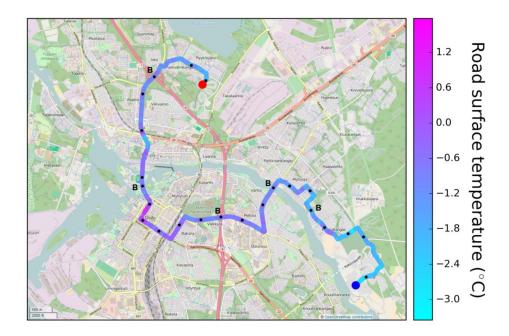
Figure 1. Road surface temperature along the bus route on 8<sup>th</sup> December 2015, 16:16-16:57 local time. The red and blue dots show the start and end points of the route, respectively. The black dots indicate the selected forecast points. The locations of bridge points are marked as "B"
