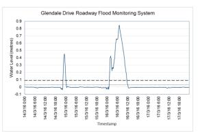
Figure 6: Radar water level data (14/03/16 00:00 to 18/03/16 00:00) measured by the Glendale Drive Roadway Flood Monitoring System.
