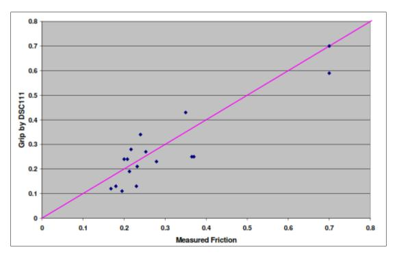
Figure 1 – Correlation between DSC111 Grip value and measured friction
